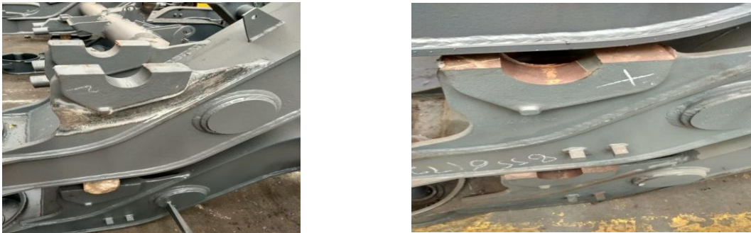
Fig.4 (a) control arm before cutting by machine and(b) control arm with improper depth of cutting
