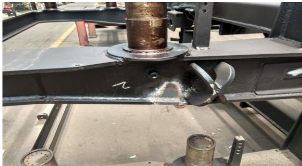
Fig. 8 Distortion in guide of bogie frames
