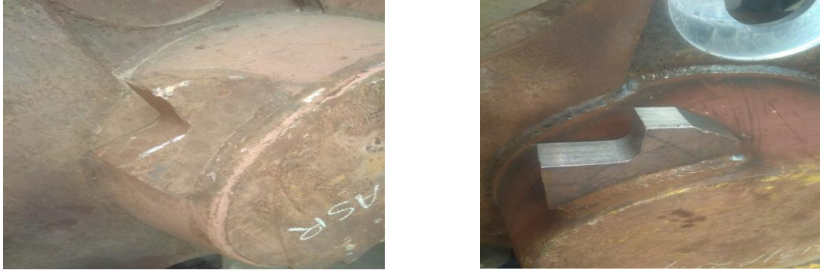
Fig. 3 (a) Mating block before machining and (b) Mating block after machining
