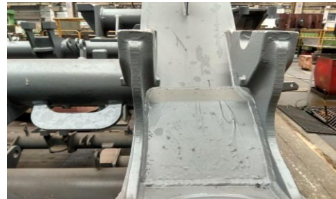
Fig.5 (a) Gap between control arms and (b) Gap between control arms after rectification
